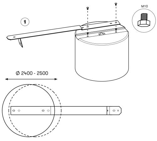
6 x HopOp 500 attach to the arms of the B14 bracket using the M10 bolts included as shown above. Two possible positions allow for a total diameter of either 2.40m or 2.50m.
