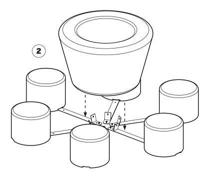
Once the 6 HopOp 500 units are mounted on their individual fittings, position them in a star formation and lower the Loop Cone part over the star to gather the vertical flanges inside Loop Cone. Now they may be pushed into position and bolted to the six brackets (see page 06).
