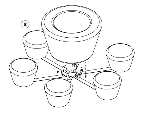
Once the 6 Loop Up units are mounted on their individual fittings, position them in a star formation and lower the Loop Cone part over the star to gather the vertical flanges inside Loop Cone. Now they may be pushed into position and bolted to the six brackets (see page 06).
