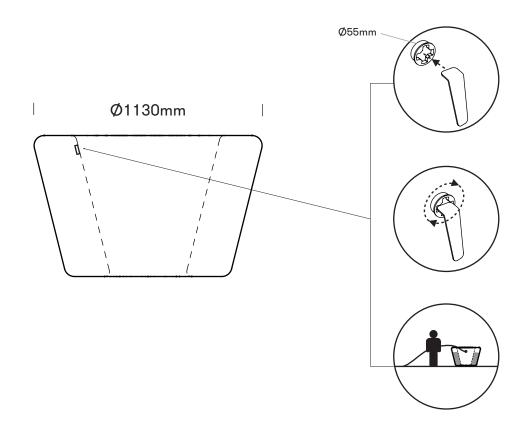
Loop Cone (22 kg) + water filled to the filling cap (305 liters of water) ~ 327 kg
