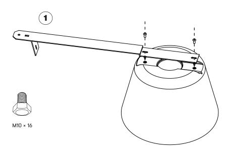
6 x Loop Up attach to the arms of the B14 bracket using the M10 bolts included as shown above. Two possible positions allow for a total diameter of either 2.40m or 2.50m.
