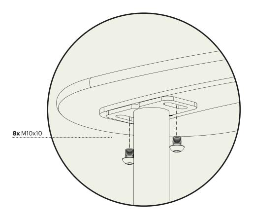
**Fastening of the seat**Use M10x10 bolts to fasten the seat to all four legs.
