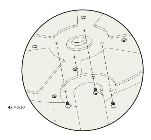
**Fastening of the table**Use M8x10 bolts to fasten the tables to the center tube.
