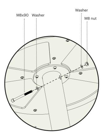
**Fastening of the disc**Use M8x90 bolt, nut and washer to fixate.
