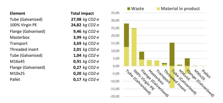
\*) The values presented here, is total emission pr element (incl. Material, production, transport, Waste)
