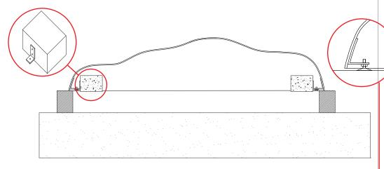
3) Prefabricated concrete blocks are mounted on the 5 internal angles with bolts and nuts. The concrete blocks are wedged up while they are mounted.
