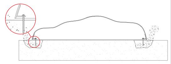
3) A number of threaded rods (corresponding the number of dug holes) is mounted in the internal angles and the StarFish is placed over the holes. The holes are filled with concrete (strength 12).
