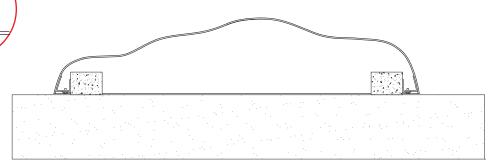
4) The elevation and the wedges for the concrete blocks are removed. The Starfish is fixed and ready for use.
