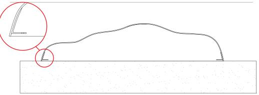
1) StarFish comes with 5 fixed stainless steel angles with Ø14mm holes. Tape markings on the outside of the StarFish indicate the locations of the angles.
