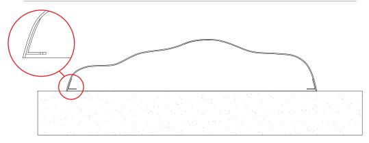
1) StarFish comes with 5 fixed internal angles (stainless steel) with  $\emptyset$ 14mm holes. Tape markings on the outside of the StarFish indicate the locations of the angles.
