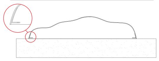
1) StarFish Mini comes with 4 fixed internal angles (stainless steel) with Ø14mm holes. Tape markings on the outside of the StarFish Mini indicate the locations of the angles.
