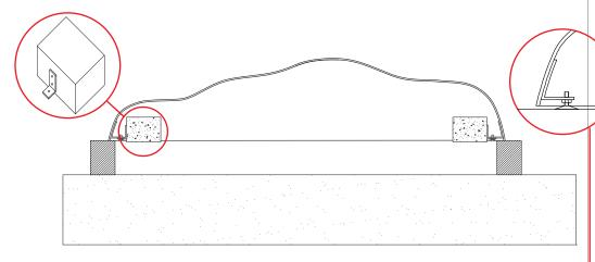
3) Prefabricated concrete blocks are mounted on the 4 internal angles with bolts and nuts. The concrete blocks are wedged up while they are mounted.
