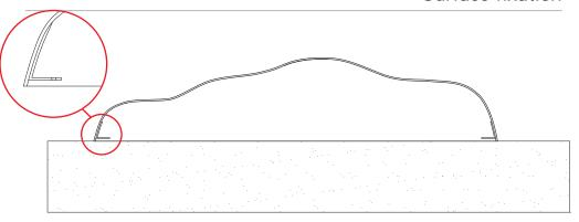
1) StarFish Mini comes with 4 fixed stainless steel angles with Ø14mm holes. Tape markings on the outside of the StarFish Mini indicate the locations of the angles.
