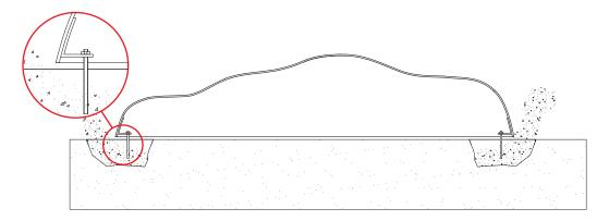
3) A number of threaded rods (corresponding the number of dug holes) is mounted in the internal angles and the StarFish Mini is placed over the holes. The holes are filled with concrete (strength 12).
