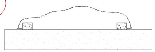
4) The elevation and the wedges for the concrete blocks are removed. The Starfish Mini is fixed and ready for use.
