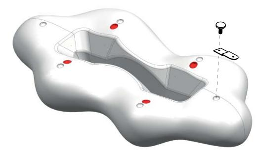
Each bracket is mounted to the bottom of Lava with supplied M8 bolts/feet.
