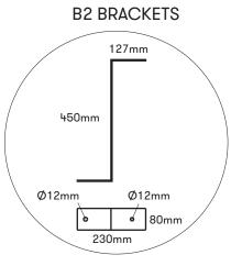
Each bracket is mounted to the bottom of Lava with supplied M8 bolts/feet.
